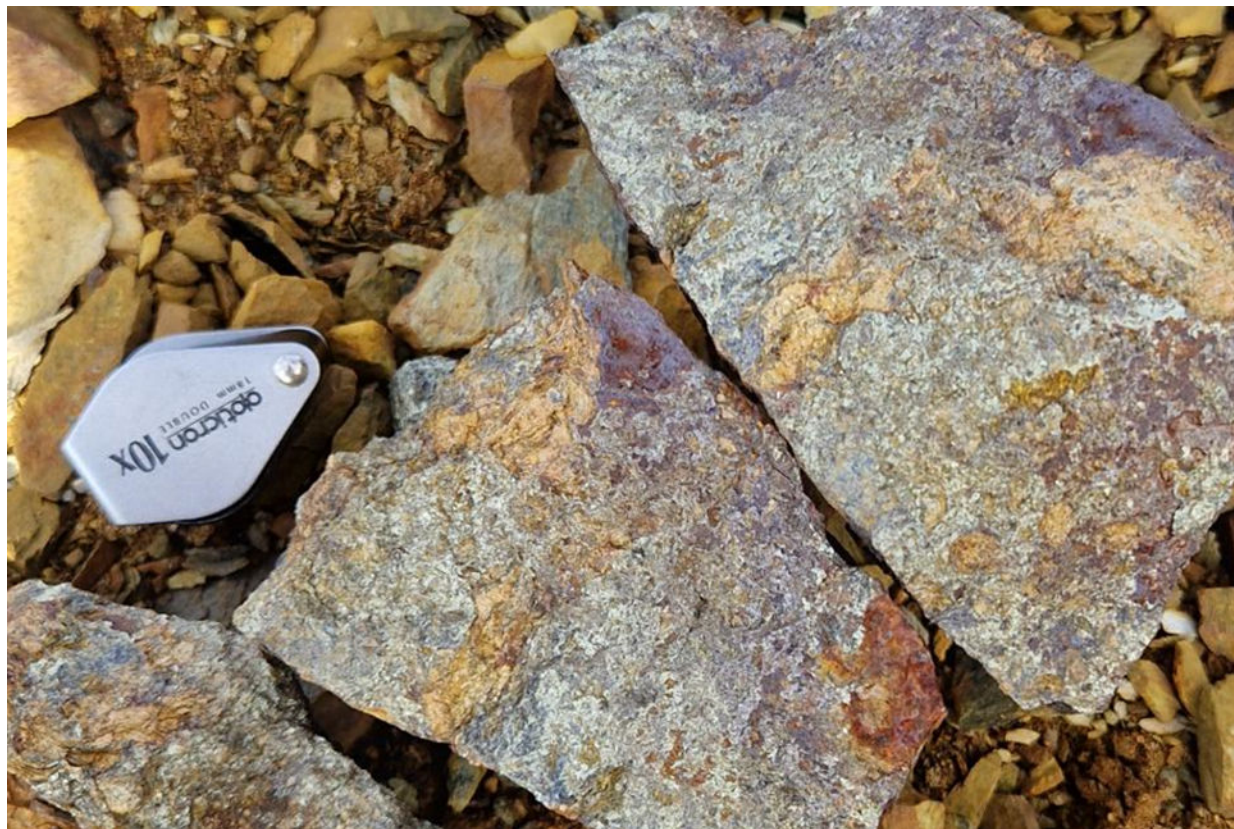
Photo 6: Sample D125056, Rock-chip sample taken from a dump in the Birtavarre area, containing 10.52% Cu. Brecciated massive sulphide containing chalcopyrite>>pyrrhotite.
