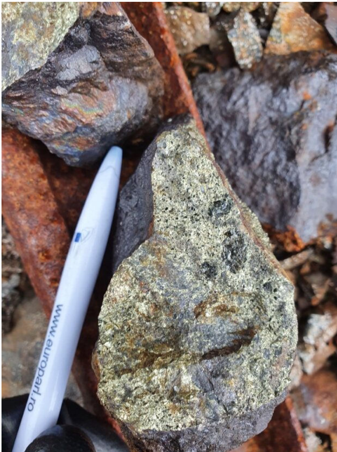
Photo 2: Sample D125040 containing 7.77% Cu, from the Indre Gressdal target
