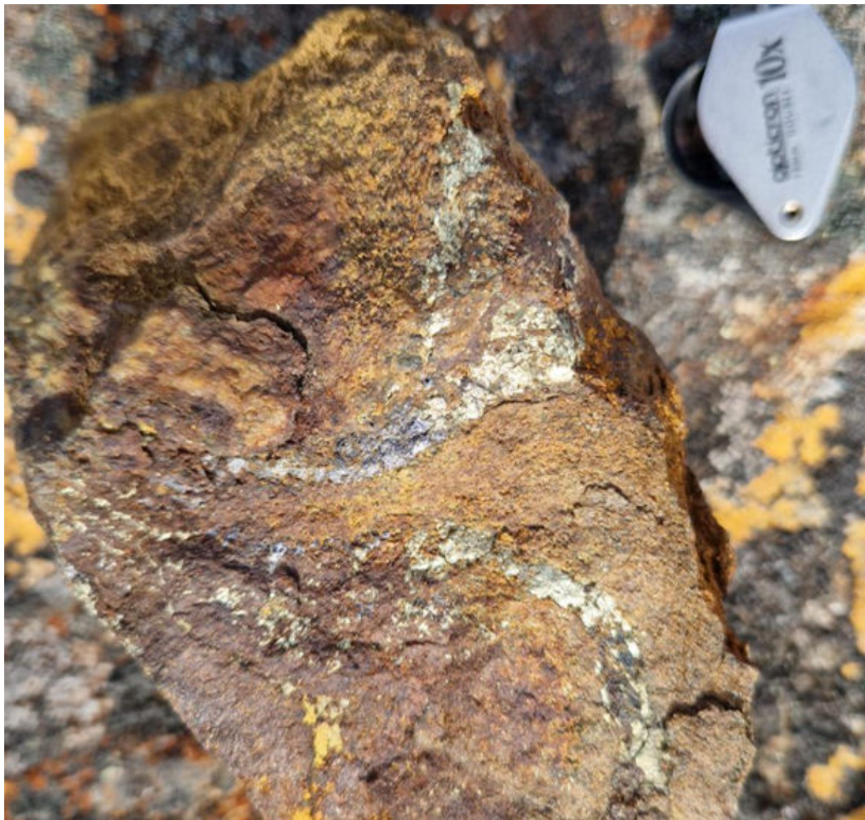
Photo 5: Sample D125049, chalcopyrite and sphalerite folded in Amphibolite containing 6.66% Cu, 2.25% Zn
